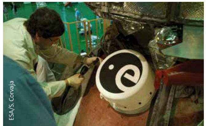
↑ Biopan exposure facility (with ESA logo) installed on the side of Foton-M3 during launch preparations in 2007
